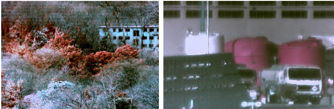
Figure 2: Photographs taken from video recorded with a 3-band SWIR video system. Assignment of SWIR bands to red green and blue display colors has been made arbitrarily. Spectral contrast can be seen in both urban and natural settings. Most of the apparent defocus in the image on the left comes from air turbulence as air is rapidly being heated by the ground. The distance to the object is over 1 mile.
